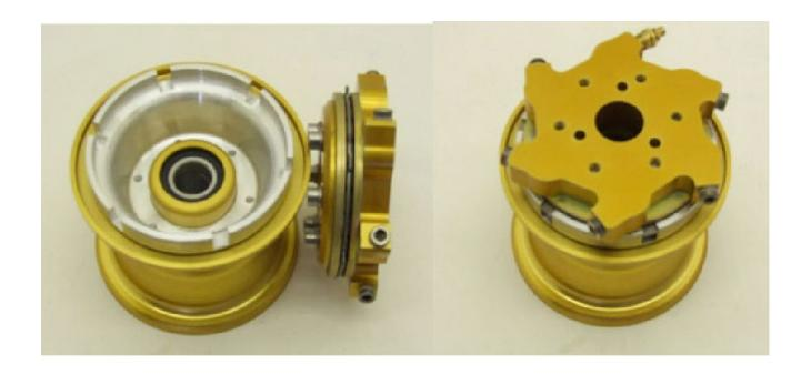
Wheel rims 4" with Rotor Brake six hydraulic pistons.
