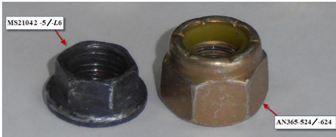
Figure 3. Nuts MS21042-5/-L6 (ANTE MOD.) and AN365-524/-624 (POST MOD.)
