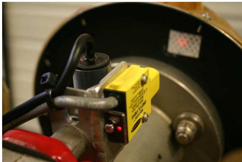
Experimental installation, showing reflective tape on spinner backing plate.
