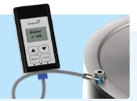
The security level Topsecure (BäderIdent®) offers an unambiguous product identification, making it an effective means against product counterfeiting and manipulation of every kind. The BäderIdent® lacquer system contains an individual code which consists of a specific fluorescent marker particle and a color. By means of a suitable analyser, you can always check on site the authenticity and integrity of your product.
